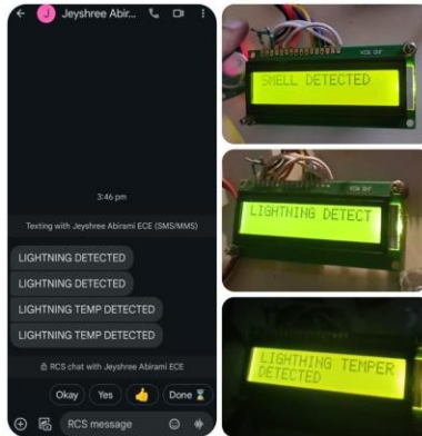
Fig 4.4 Lightning Monitoring and Obstacles Detection
